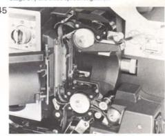
46 Unscrew the knob 46a securing the exciter lamp cover and pull the cover carefully away from the projector.
