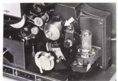
The magnetic head should occasionally be taken out (Stage 60) and lightly brushed to remove any particles of magnetic oxide. Do not attempt to remove obstinate accumulations of oxide from the head with any tool or fluid. This is a delicate component, adjusted in the factory to a high degree of precision. If it cannot be cleaned by gentle brushing, ask your dealer to do the job.
