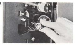
54 Grasping the retaining clip and lamp base between finger and thumb, raise the clip until it clicks into the notch in the lamp base.
