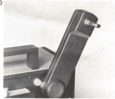
11 Raise the rear spool arm until it locks with a click at the "7 o'clock" position (this is a special position not used in normal operation). Press the release button 11a and raise the arm further. Release 11a and continue to raise the arm until, when horizontal, it again locks with a click.
