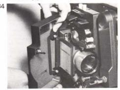
35 Pull the front of the lens barrel towards you to open the film gate 35a. Pull down the lower access door 35b.
