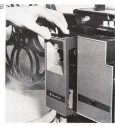
52 Remembering that if the lamp has just failed it will be hot, disengage the retaining clip 52a by firm downward pressure and leave it hanging free.
