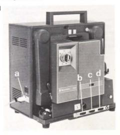
Pull down the rear flap and remove the power lead. Do not connect the power lead to the mains until you reach Stage 7. This projector is suitable only for alternating current (AC) supplies of 50Hz or 60Hz and may be seriously damaged if connected to direct current (DC) supplies. If you have any doubt about whether your supply is AC or DC, seek the advice of a competent electrical contractor or your local electricity office before connecting the projector to the mains.
