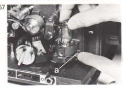
58 Fit the ring of the new lamp over the three studs — there is only one position in which this can be done — and rotate the lamp until the studs are at the narrow ends of the slots in the ring. Pull the securing lever 58a all the way back to its running position. Replace the exciter lamp cover, reset the main power switch to "on" and close the main access door.
